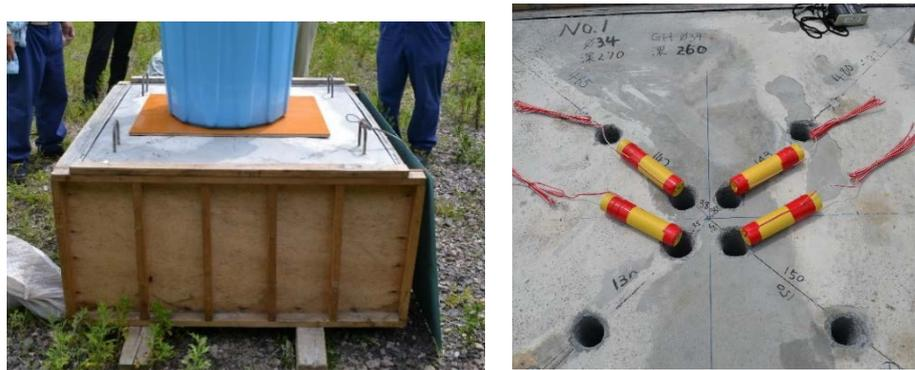
Figure 3. SPC agent insertion into large concrete test pieces
