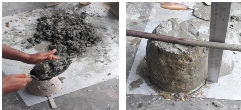
Fig. 2. Slump test (a) mould preparation (b) slump value measurement
