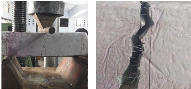
**Fig. 11.** Beam failure and fibre bridging
