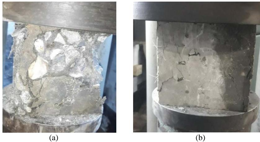
Fig. 8. Failure pattern (a) normal concrete (b) fibre reinforced concrete
