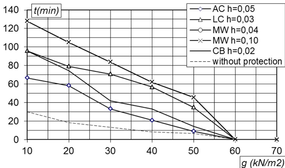
**Fig.2** Dependence of the bearing capacity of steel concrete slab upon the type of thermal protection
