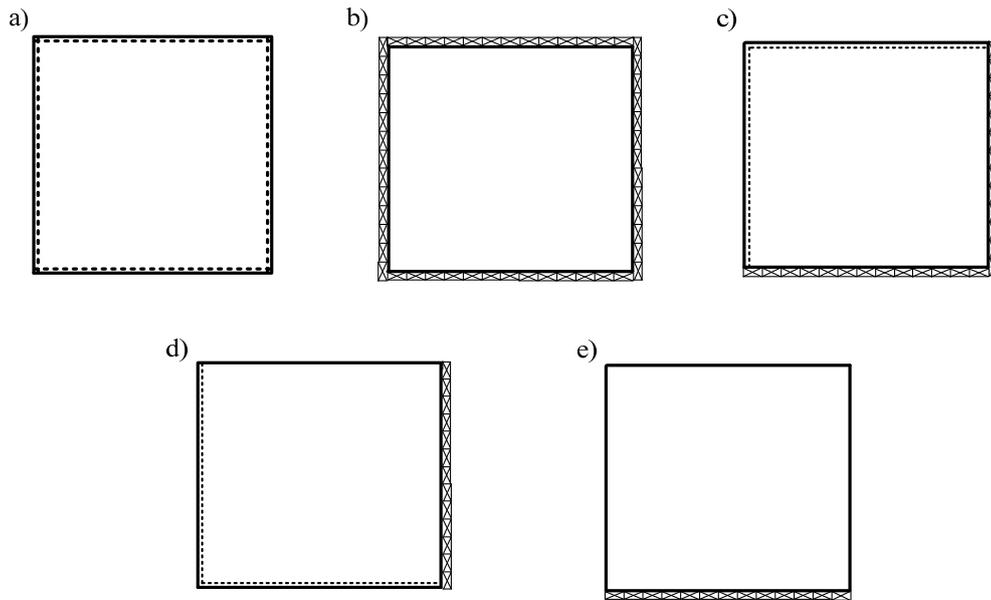
**Fig.3 Schemes of supporting slabs: a) with hinge-supported edges; b) with fixed edges; c) 2 fixed edges, 2 hinge –supported edges; c) one fixed edge; d) plate console, that is one edge is fixed, and the rest are free.**
