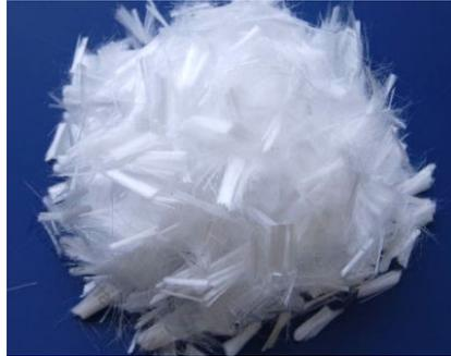
**Fig.6 Polypropylene fibrous**
