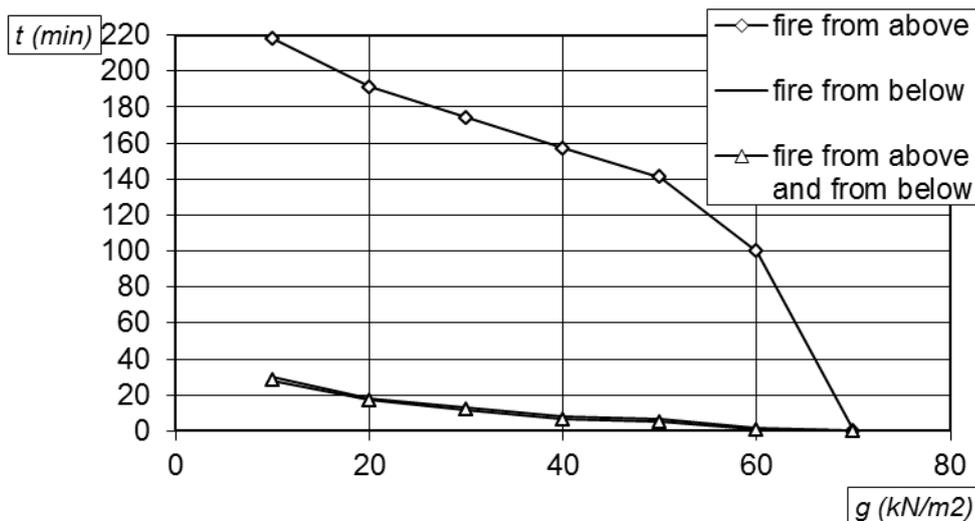
**Fig.1** Dependence of the bearing capacity of steel concrete slab upon the circuit thermal effects
