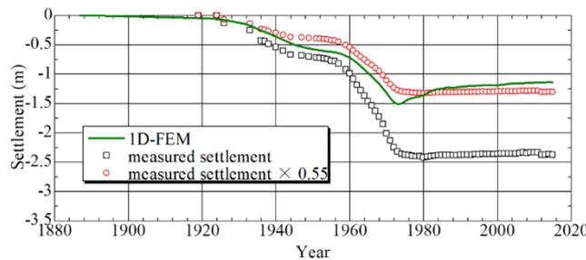
Fig. 6. Comparison of calculated compression and measured settlement
