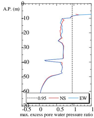
Fig. 11. Max. excess pore water pressure ratio distribution in 2011 (Taisho Kanto earthquake)
