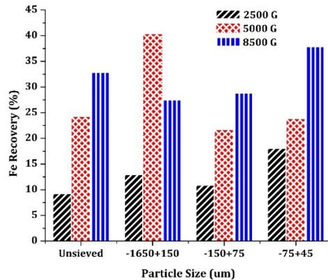
Figure 8. Iron recovery in various size fractions at different magnetic intensities
