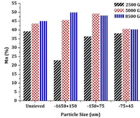
Figure 5. Manganese percentage in various size fractions at different magnetic intensities
