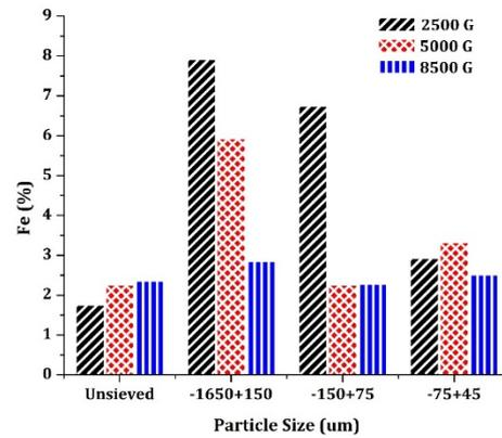
Figure 7. Iron percentage in various size fractions at different magnetic intensities
