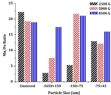
Figure 9. Manganese/Iron ratio in various size fractions at different magnetic intensities
