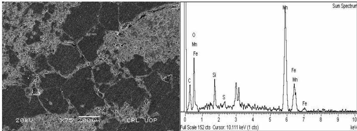
Figure 3. SEM and EDX of raw manganese ore
