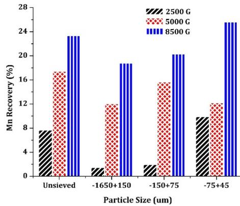
Figure 6. Manganese recovery in various size fractions at different magnetic intensities
