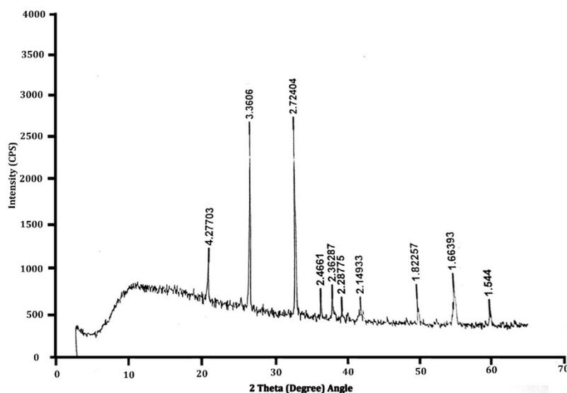
Figure 2. XRD analysis of raw manganese ore
