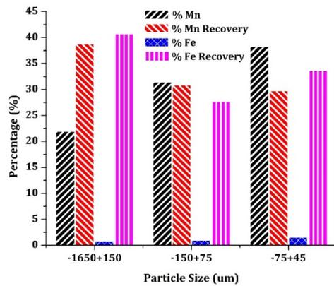
Figure 4. Manganese and Iron recoveries in various size fractions during wet sieving
